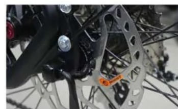
Bremsscheibenadapter am Bicycles EXT 500 LTD
